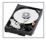
**Hard Disk Drive (HDD)** is a long-term storage device used to store programs, documents, and files. HDD stores data on mechanical platters. It uses a moving read/write head to read and write data to the platters.
