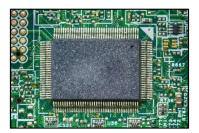
**Read Only Memory (ROM)** stores data that can be read and used but not changed. ROM chips store instructions that control the basic functions of the computer. These instructions remain in ROM regardless of whether the power is on or off.
