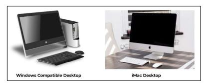
An all-in-one computer is a special kind of computer that has everything you need in one place. Its appearance is like a regular computer monitor, but instead of just a screen, there are important parts inside the monitor like the brain (processor), memory, and storage. The complete computer is in a single piece. These computers are designed to be energy-efficient, which means they use less electricity than regular computers.
